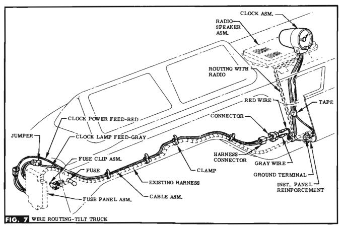
\$75P 15 INSTALL FUSE CLIP & FUSE INTO RECEPTACLE IN FUSE PANEL ASM, MARKED "GL. BOX LP." & PLUG IN RED WIRE CONNECTOR (POWER FEED).SEE FIG. 5, 6, 7 OR 8.
