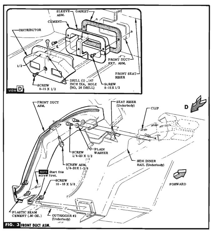
STEP 15 CEMENT GASKET TO SLEEVE & SLIDE SLEEVE THRU OPENING IN SEAT RISER & INTO FRONT DUCT EXTENSION. ATTACH WITH SCREWS (IN BAG A). SEE VIEW D.
