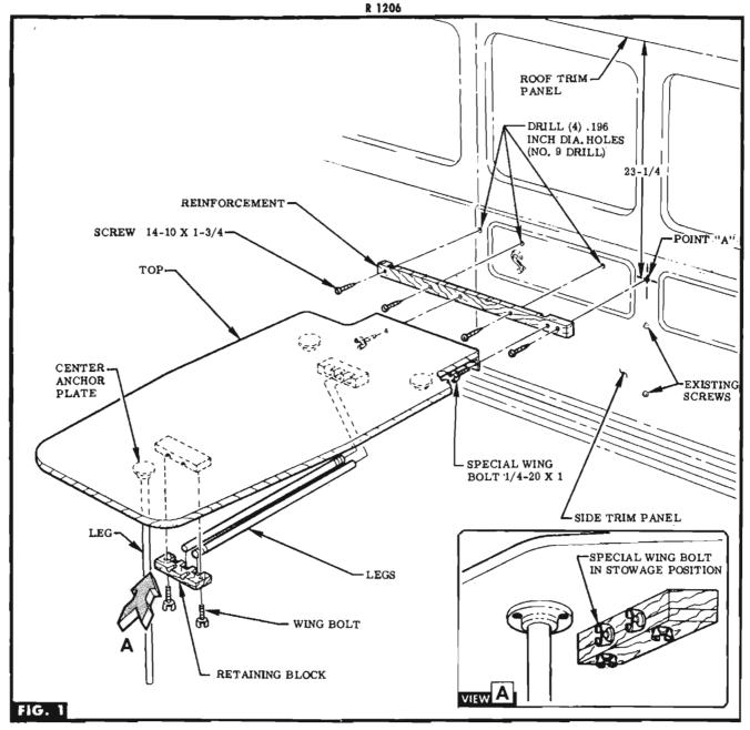
STEP 1 LOCATE POINT "A" & DRILL HOLE THRU SOFT TRIM PANEL (IF EXISTING) & METAL SIDE TRIM PANEL. HOLE IS TO BE IN ALIGNMENT WITH EXISTING SCREWS. SEE FIG. 1.
