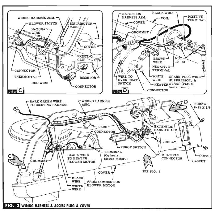
STEP 12 PLUG HARNESS CONNECTORS ONTO BLOWER SWITCH & RESISTOR, SEE VIEW C.
