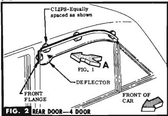
NOTE Deflectors are stamped to show position LF for Left Front, RF for Right Front, etc.
