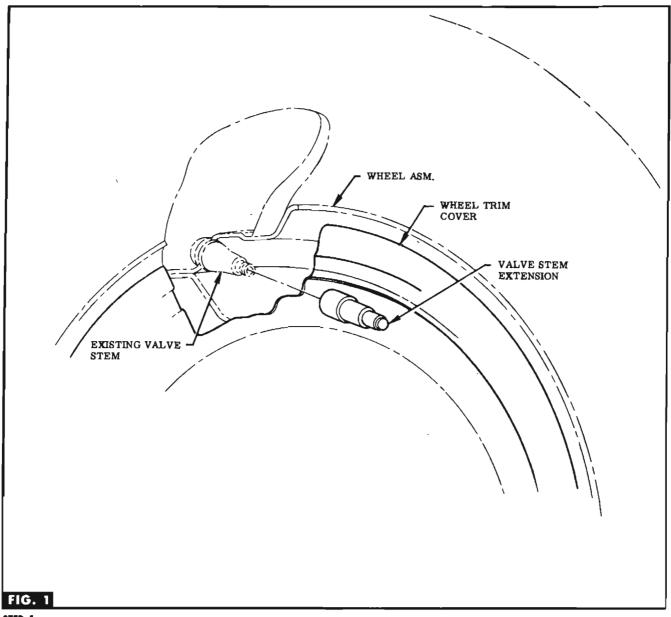
**STEP 1** REMOVE EXISTING VALVE CAP & INSTALL PROVIDED EXTENSION TO VALVE STEM, SEE FIG. 1.
