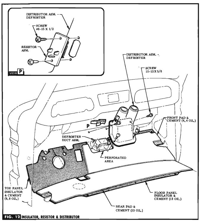
\$16P 63 REMOVE EXISTING FLOOR MAT & CEMENT PROVIDED PADS TO UNDERSIDE OF FLOOR MAT. CUT OUT PERFORATED AREA. SEE FIG. 1.
