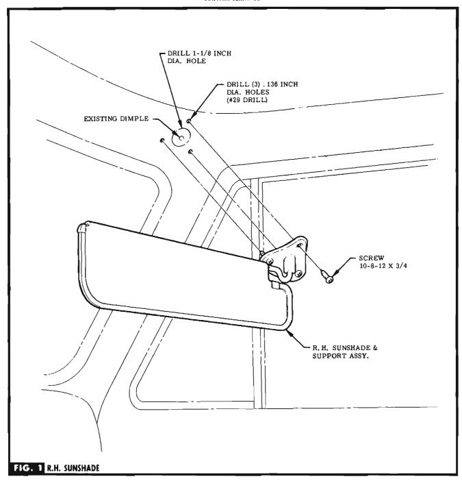
**STEP 1** LOCATE EXISTING DIMPLE & DRILL LARGE HOLE IN TRIM PANEL, SEE FIG. 1.
