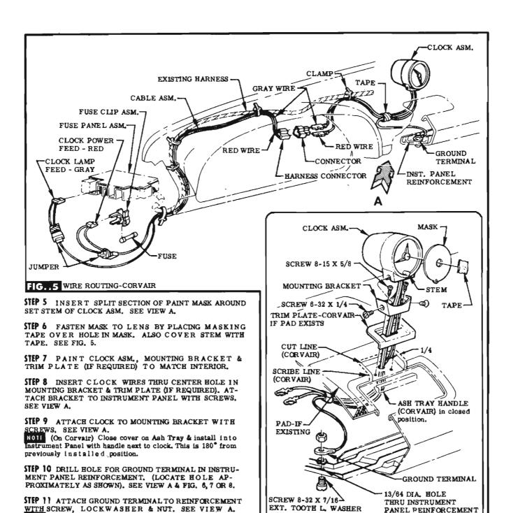
NOTE (Truck R10 & Truck Exc. Titt) Coil excess cable & clamp as shown. See Fig. 6 or 8.
