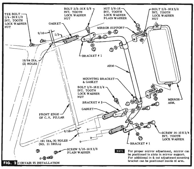
STEP 16 ON L. H. SIDE ONLY, REMOVE & DISCARD EXISTING MIRROR & ATTACHING PARTS. PLUG HOLES WITH PARTS PROVIDED, SEE FIG. 2.
