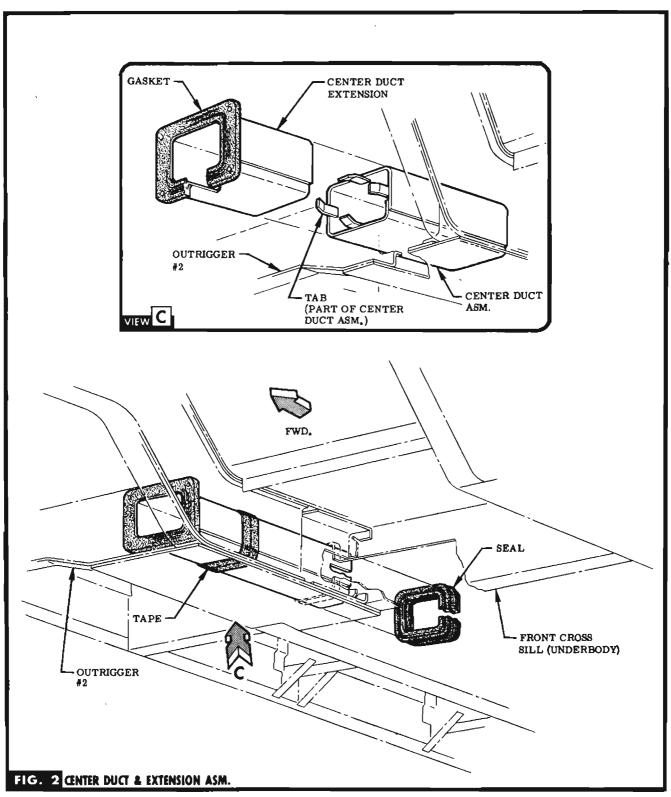
STEP  $\mathbf{9}$  Install gasket onto center duct extension. See view  $\mathbf{c}_{\star}$
