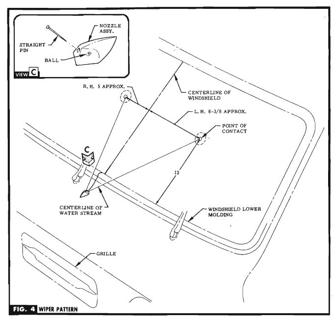
STEP 11 TEST SYSTEM TO INSURE CORRECT INSTALLATION & DETERMINE LOCATION OF POINT OF CONTACT FOR WATER STREAM, SEE FIG. 4.
