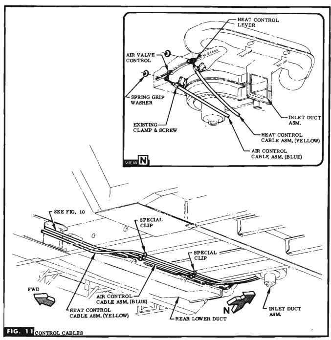
STEP 57 INSTALL CLIPS (IN BAG B) TO INTERMEDIATE & REAR CROSSMEMBERS ALONG SIDE DUCT SECURING SCREWS, SEE FIG. 11.
