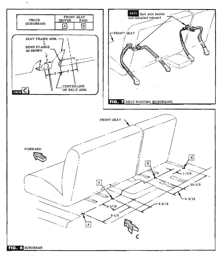
STEP 2 BEND SEAT FRAME ASM. FOR LEFT HAND INBOARD BELT. SEE FIG. 8 & VIEW "C".
