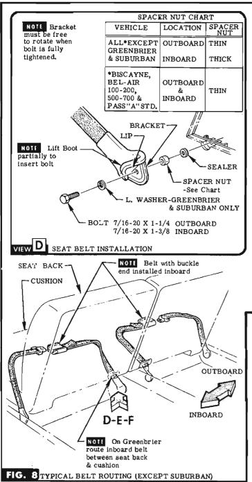
SEAT . BACKING OR REINF. Note Cut between existing "V" slits in fabric TRIM PROTECTOR SCREW ALL EXCEPT BUCKET SEAT, GREENBRIER & SUBURBAN FRONT SEAT BACK SEAT CUSHION REAR CUT-SEE VIEW E EXISTING FRONT SLOT 2 DOOR MODELS EXCEPT BUCKET SEATS, GREENBRIER & SUBURBAN NOTE Belt with buckle end installed inboard
