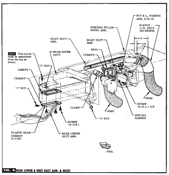
STEP 28 REMOVE FILLER PANEL ASM, & ATTACHING PARTS & RETAIN,
