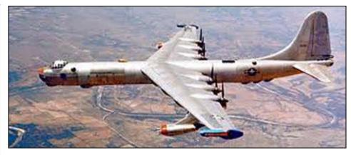
A Convair B-36 Peacemaker Bomber in flight. Note the six rear-facing piston engines and the two forward-facing sets of double jet engines
