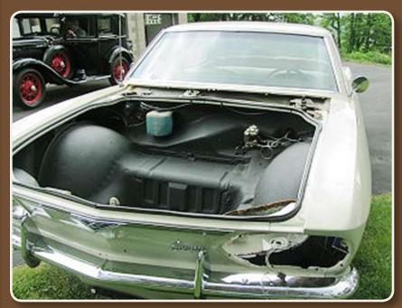
Jim Heatherington's Corvair after Don Cekus removed the trunk lid. Notice that there was no damage to the windshield even though the Corvair was traveling at about 50 miles per hour when the trunk lid suddenly blew open. However, along with the hinges, there was damage to the cowl just in front of the windshield.
